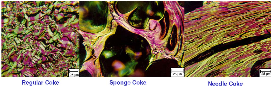
Fig. 1. Various forms of coke: microscopic pictures in polarized light (by courtesy of Prof. Crelling [2]).
